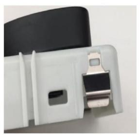
Align the circuit board plunger and key guide as shown below to the LOCK position.
