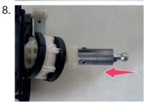
Slip the new end on the base of the shifter & screw 2 screws.
