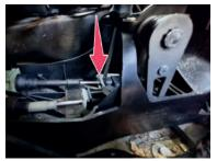
Insert small screwdriver into second shift cable lock and gently twist
