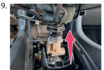
Pull up gear stick to make spring lock
