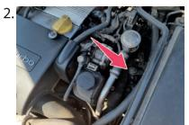
Find gear selector on the right side of the engine
