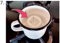
To make it easier to put a new bushing on, we need to warm it up to make it more plastic. Boil the water and put the sleeve in the pot.
