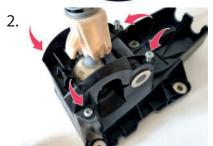
Remove the bolts and release the shift cable from the jack pin.
