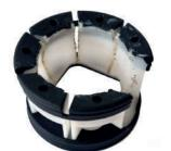
Replace the worn selector bushing which has a loose one. This can cause play in the gearshift lever.
