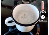
Place the new bushing in boiling water for about 10-12 minutes
