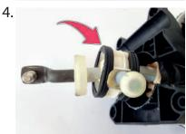
The seat of the old lever selector bushing that we are replacing.
