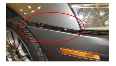
Remove the headlights by removing 3pcs of 10mm (on facelift 2pcs 10mm & 1pc 8mm) hex screws on each headlight and then pull/lift forward so you can disconnect the electrical connector from the headlight and then remove headlight from vehicle.
