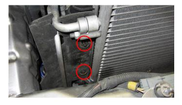
Remove the power steering pipe bracket by removing the 10mm hex head screw, turn it upwards and pull loose.
