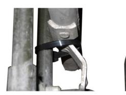
18. Remove the 2pcs Torx T25 screws that attaches intercooler to radiator (one on each side of intercooler).
