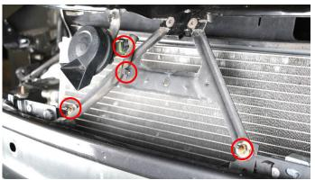
9. Remove the radiator support by removing 8pcs of 10mm (on facelift 6pcs) hex head screws.
