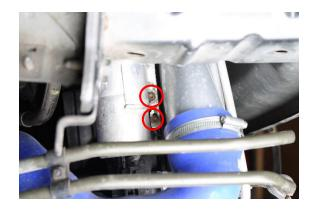
Loosen both hoses from intercooler by loosen hose clamps (with a 7mm hose clamp screwdriver or 7mm hex socket) and pull them off the intercooler connections.
