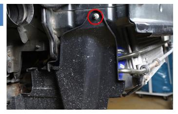
11. Remove the air guide from the top of the intercooler by pulling it upwards.
