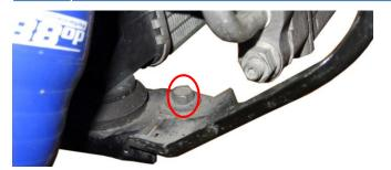
Remove the 10mm hex head screw that attaches power steering pipe clip to bracket.
