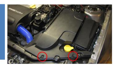
2. Remove the 4pcs 8mm hex head screws in each front inner fender.
