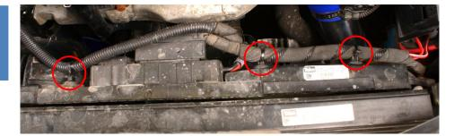
Remove 2x T25 Torx screws in top of each corner of the fan shroud.
