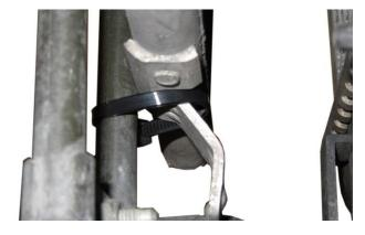
Loosen both hoses from intercooler by loosen hose clamps (with a 7mm hose clamp screwdriver or 7mm hex socket) and pull them off the intercooler connections.
