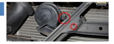
Remove the two Torx T25 screews that secures the air inlet pipe to the radiator support.
