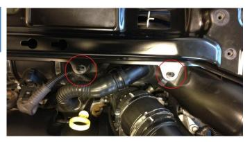
Remove the radiator support by removing 8pcs of 10mm (on facelift 6pcs) hex head screws on top of it and 2pcs of 10mm hex head screws in the bottom of the cross member.
