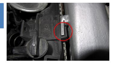
22. Attach the intercooler to the radiator with the two included 5x25 Torx T25 plastic screws . One on each top end of the intercooler.
