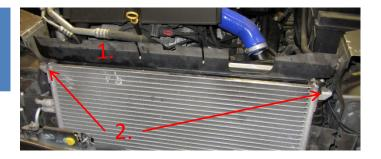
Remove the air guides on both sides of the intercooler by gentle pry out the tabs in the washer and then remove from intercooler pin. Remove air guides from intercooler.
