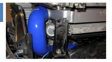
Install the hose between intercooler outlet and intercooler pipe.
