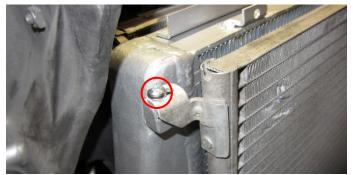
Install the upper air guide on the front side of the bracket on top of the intercooler using three included 4x16mm self drilling metal screws (not on included parts picture).
