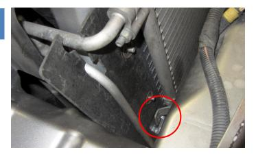
**25.** Fasten the AC condenser to the intercooler with the two included M5x16 Torx T25 screws. One on each side of condenser.
