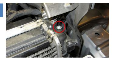
18. Remove the intercooler by lifting it up from the radiator slots and then carefully remove the intercooler downwards starting with the left hand side and then the rest of it according to picture.
