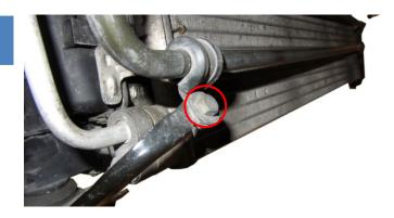
13. Remove the power steering pipe bracket by removing the 10mm hex head screw, turn it upwards and pull loose.
