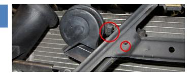
Remove the radiator support by removing 8pcs of 10mm (on facelift 6pcs) hex head screws on top of it and 2pcs of 10mm hex head screws in the bottom of the cross member.
