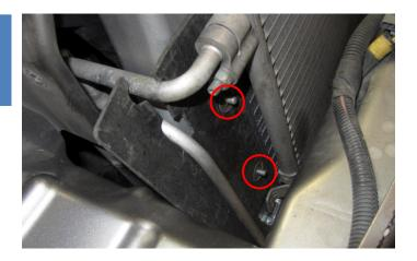
24. Install the AC condenser on the new intercooler by inserting the tabs in the intercooler condenser brackets.
