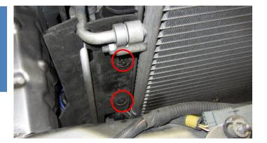
**12.** Remove the 10mm hex head screw that attaches power steering pipe clip to bracket.
