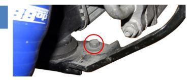
14. Loosen the 10mm hex nut just a bit, the remove the 10mm hex head screw from the bracket and then turn the bracket out from the car.
