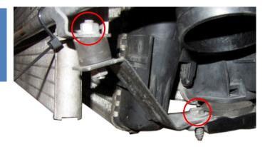
15. Lift the AC condenser upwards from its slots in the intercooler and tie it toward bumper beam as much forward as possible.
