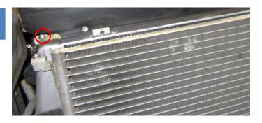
Install the OEM air guides on each side of the intercooler using the tab washers removed in step 11.
