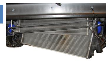
To install the intercooler on a 4 cylinder model 9-3 the lover brackets needs to be removed. Drill the 2pcs of rivets on each bracket heads using a 8mm drill and drill only about 3mm (1/8") deep. Take car to not drill to deep. If you drill about 10mm deep you might cause a leak in the core.
